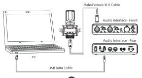
2 Connection for audio device without built-in 48V phantom power:
